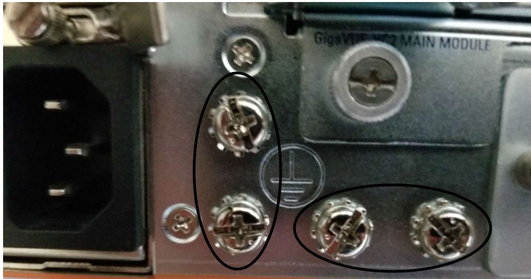
Figure 4-1: Grounding Points for Ground Screws (GigaVUE-HC2 Shown)
